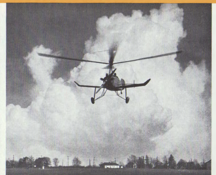
Constant support independent of engine or forward speed permits almost vertical descent with the engine idling, or stopped (right). The Pitcairn Tandem lands in the length of its shadow, with scarcely any forward roll.
