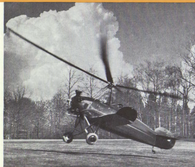
Constant support independent of engine or forward speed permits almost vertical descent with the engine idling, or stopped (right). The Pitcairn Tandem lands in the length of its shadow, with scarcely any forward roll.
