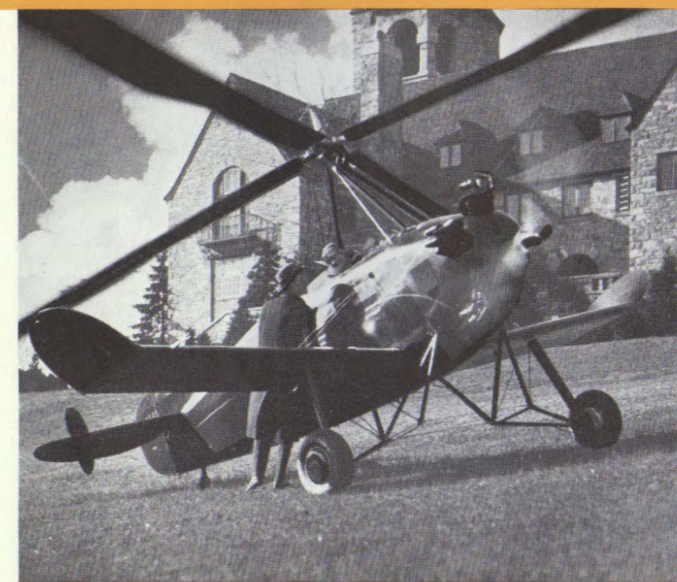
The Pitcairn Tandem, ready to leave the lawn of a country home, with engine and rotor blades started in motion. (Right) Blades have reached take-off speed as shown by the characteristic upward coning position.
